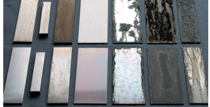
Fig. 4 Comparison of raw (top) and coated (bottom) samples after salt spray test
