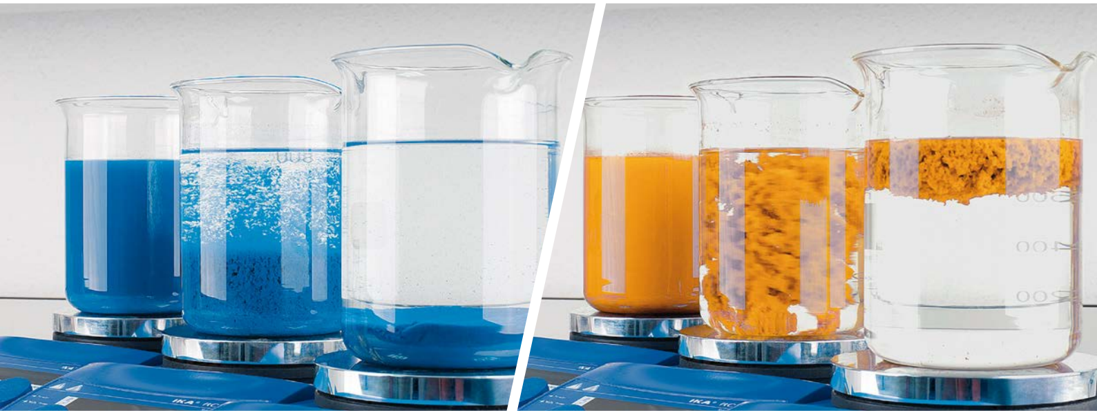
Excellent paint coagulation with Gardofloc®: for sedimentation (left) and flotation (right)
