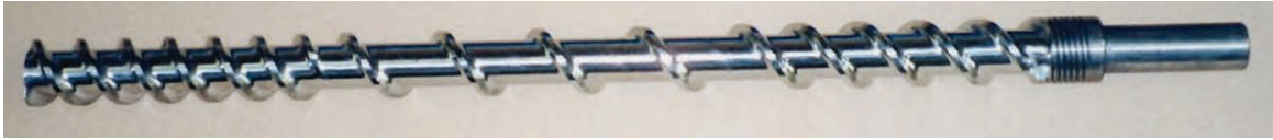
Fig. 1: Screw design of a flight progressive screw for silicone rubber extrusion
